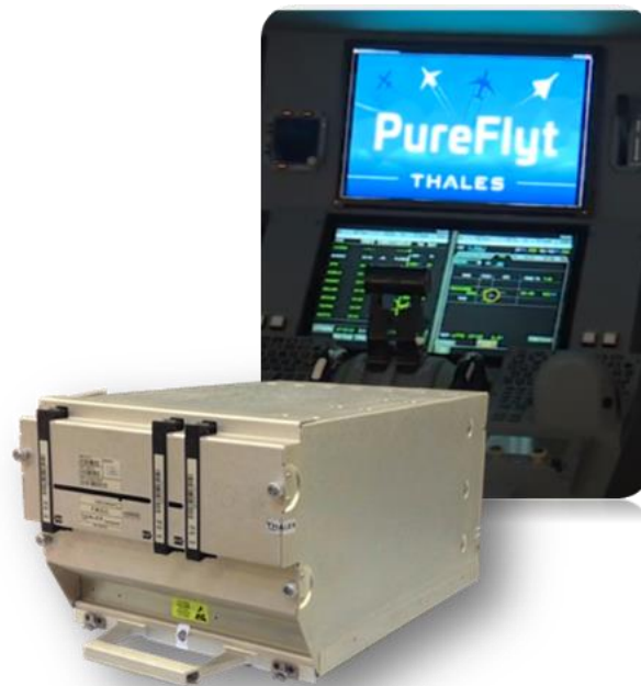
Figure 14: PureFlyt™ FMS and MFD used for DYNACAT prototype
