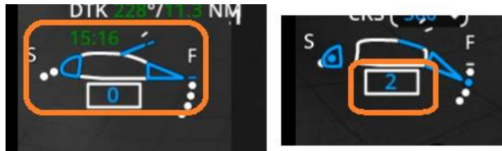
Figure 25: Display of speed brakes (left) and flaps (right) extension after bench integration
