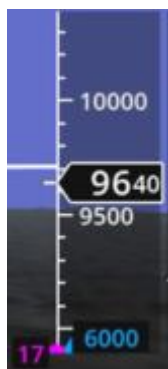
Figure 21: VDEV symbol on the PFD
