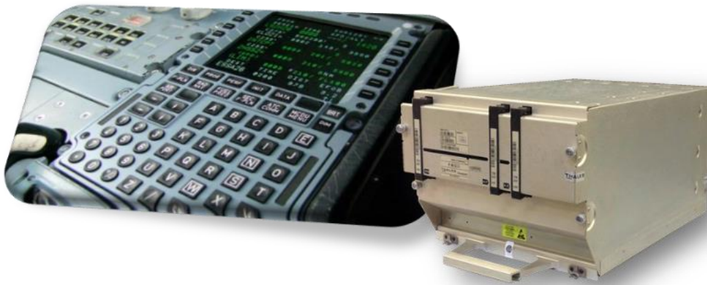
Figure 5: Flight Management System equipment
