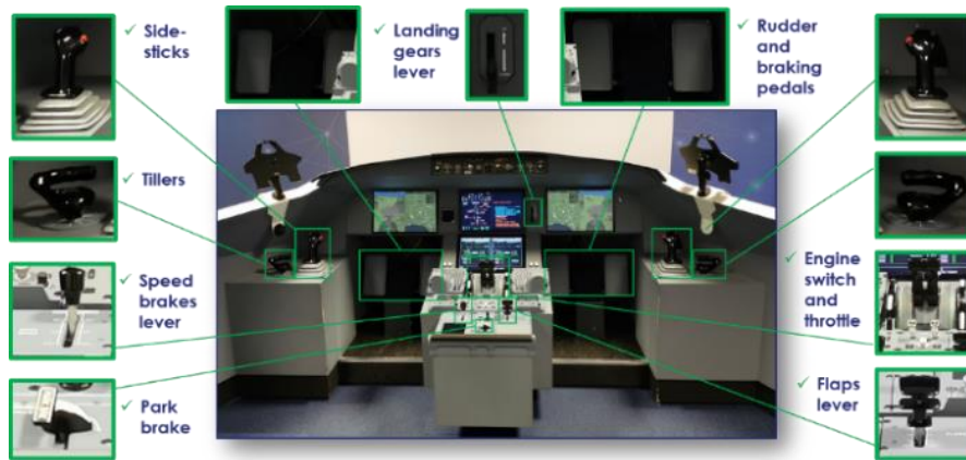
Figure 14: Focus on the Flight Control Devices
