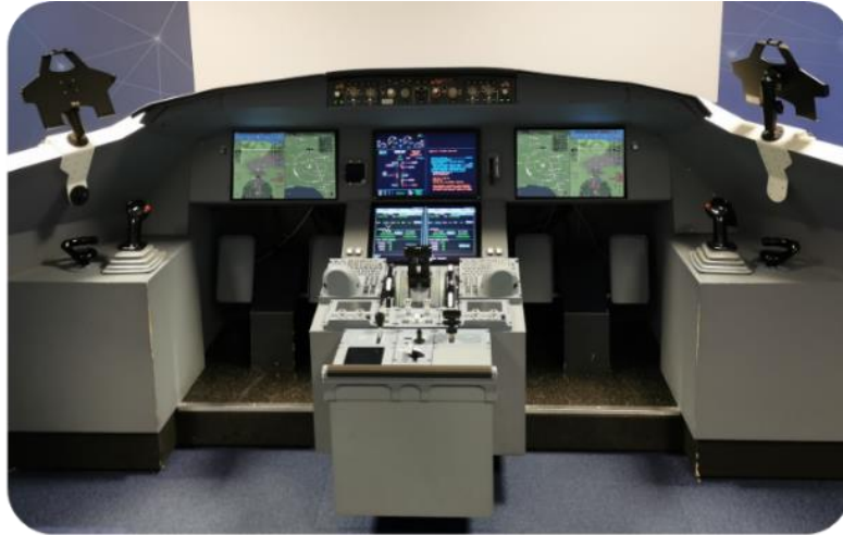
Figure 11: Flight Test Simulation bench
