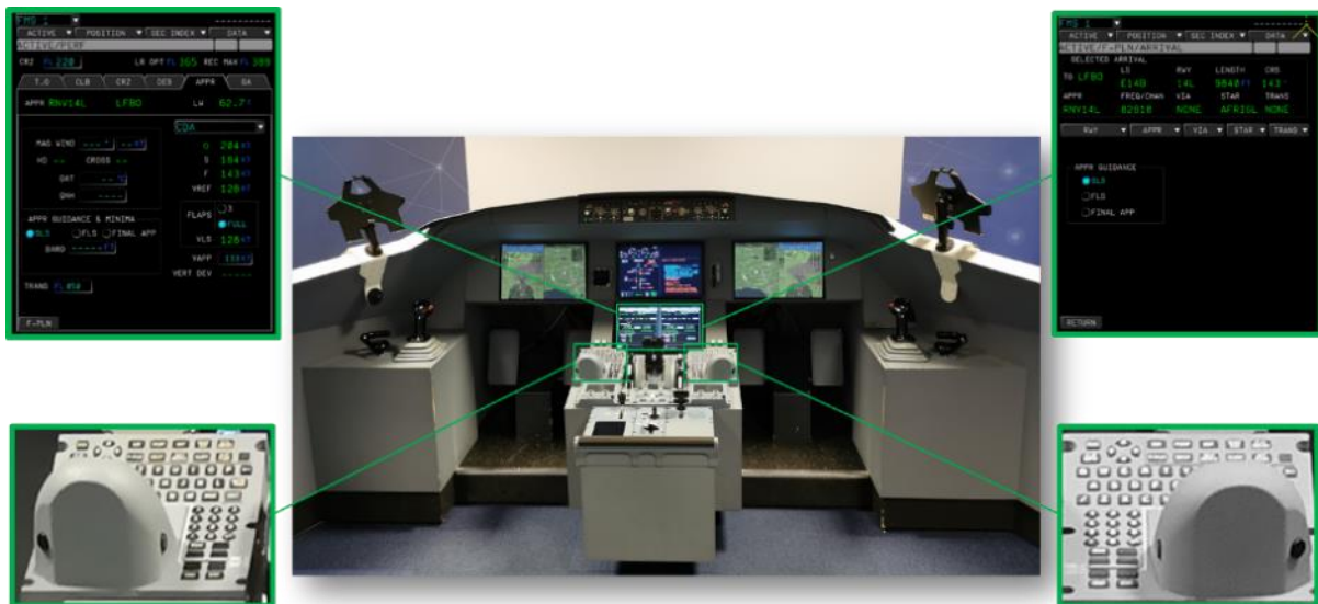
Figure 12: Focus on the Flight Management Display and interactions means (KCCU)
