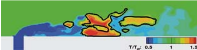
Standardised temperature distribution of an air-fuel mixture containing hydrogen after self-ignition. The black lines show the limits of the flame zones.
