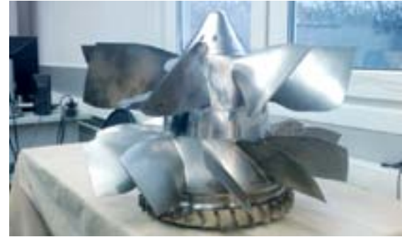
Pre-assembled and instrumented rotors of the CRTF2b contra-rotating fan
