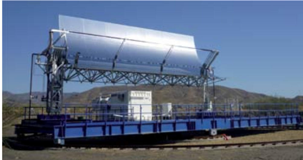
Rotatable parabolic trough test bench on the PSA
