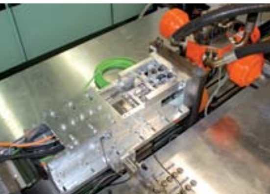
Free-piston linear generator mounted on the test bench
