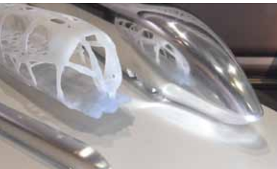
Silver objects: Wind tunnel model used to investigate side-wind stability and optimise resistance. Light-coloured framework: Design model for topology optimisation
