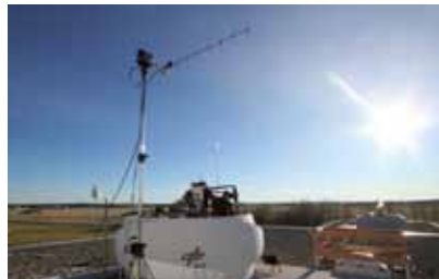
Data transmission by laser and optical terminal on aircraft (top) Optical ground station with a diameter of just 40 centimetres (bottom)
