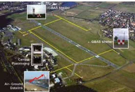
Experimental GBAS station at Braunschweig Research Airport
