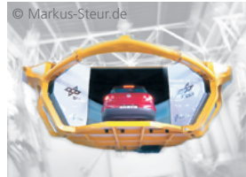
© Markus-Steuer.de DLR conducts research into driver assistance systems on its dynamic drive simulator
