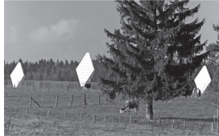
1971 VHF interferometer for measuring satellite orbits
