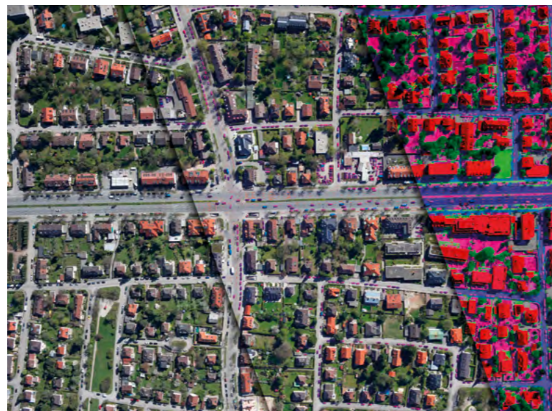
Artificial intelligence is used to classify objects in aerial and satellite images. The algorithm recognises traffic routes, vehicles and different road markings from an altitude of approximately 500 kilometres, as shown here in a scene from Munich. © EOC
