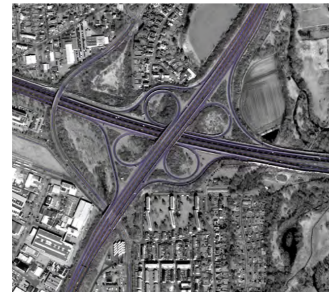
Here too, in this satellite image of a motorway junction in Braunschweig, the algorithm recognises road markings from an altitude of approximately 500 kilometres. This is valuable information for future applications such as autonomous vehicles. © EOC
