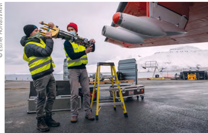
Manuel Moser and Valerian Hahn prepare the Cloud Combination Probe, an instrument for measuring water droplets and ice crystals present in clouds.
