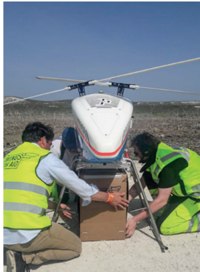
With each flight, the unmanned helicopter transported up to 25 kilograms of food, water and medicine, six kilometres over the Enriquillo salt lake, safely dropping the payload boxes on the other side.
