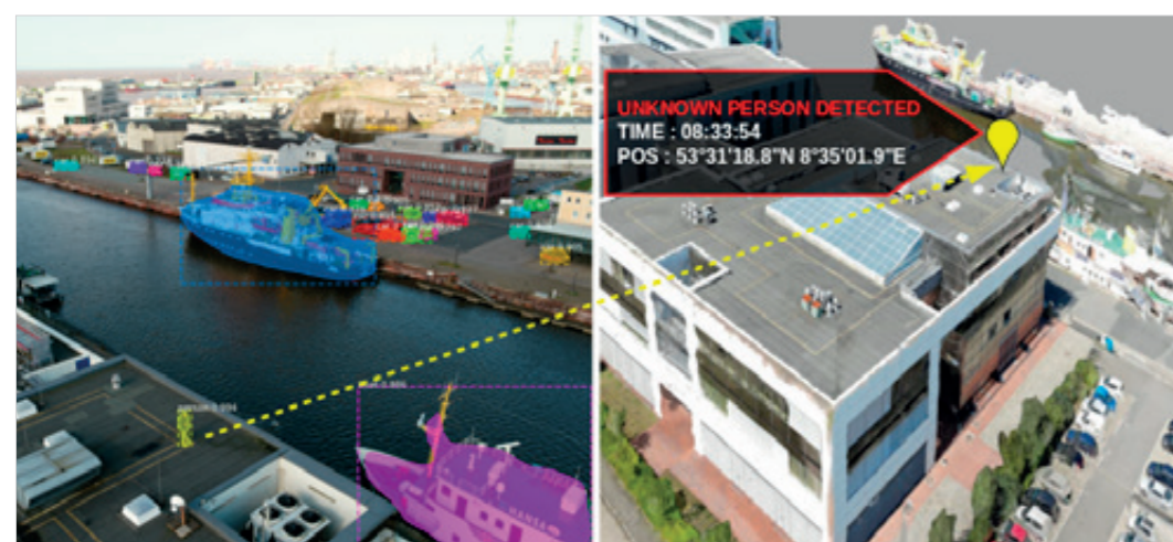
Three-dimensional, real-time image of port area in Bremerhaven. Left: Camera image with objects that have been automatically identified by artificial intelligence and colour-coded according to their shape. Right: Preliminary 3D model of the surroundings with details of the position of an unknown or unauthorised person in the area.
