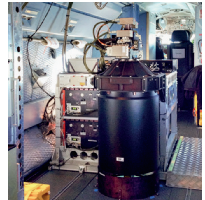
The aerosol and water vapour lidar implemented by the DLR Institute of Atmospheric Physics
