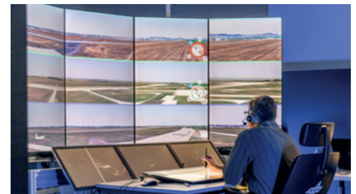
As part of SESAR, scientists at the remote tower facility at DLR in Braunschweig are conducting research into remote airport monitoring by controllers.
