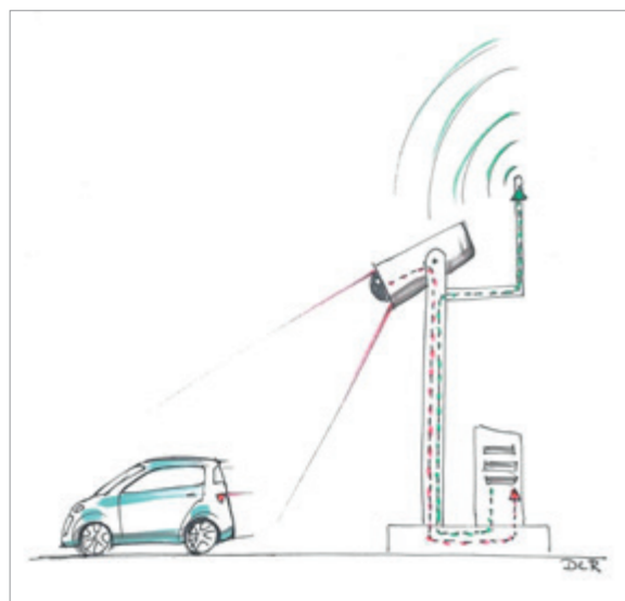
The tracking and communications technology at the edge of the test field records the speed, position and direction of travel of passing cars and lorries and transmits this information to other vehicles. This simulates the communication between vehicles.
