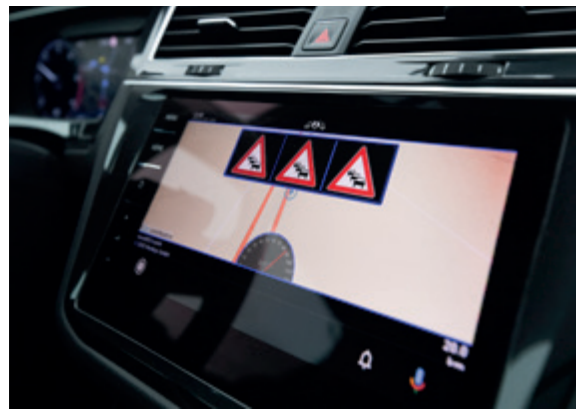
Look out: traffic jam! The communications technology warns drivers about traffic jams and accidents in real time.
