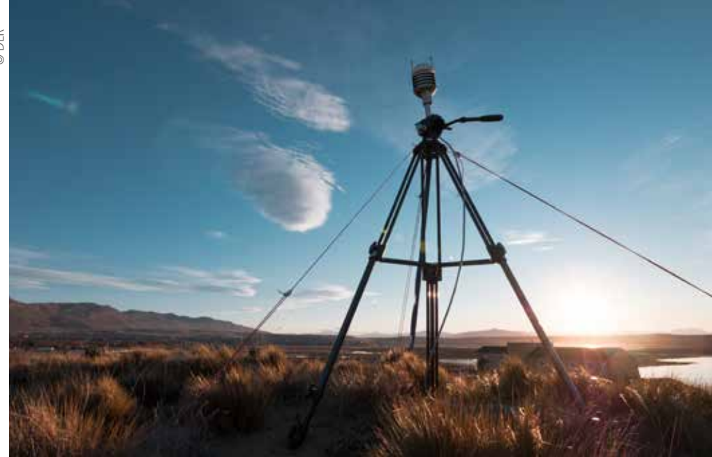
Meteorological ground station in El Calafate, operated by Ludwig-Maximilians-Universität München.
