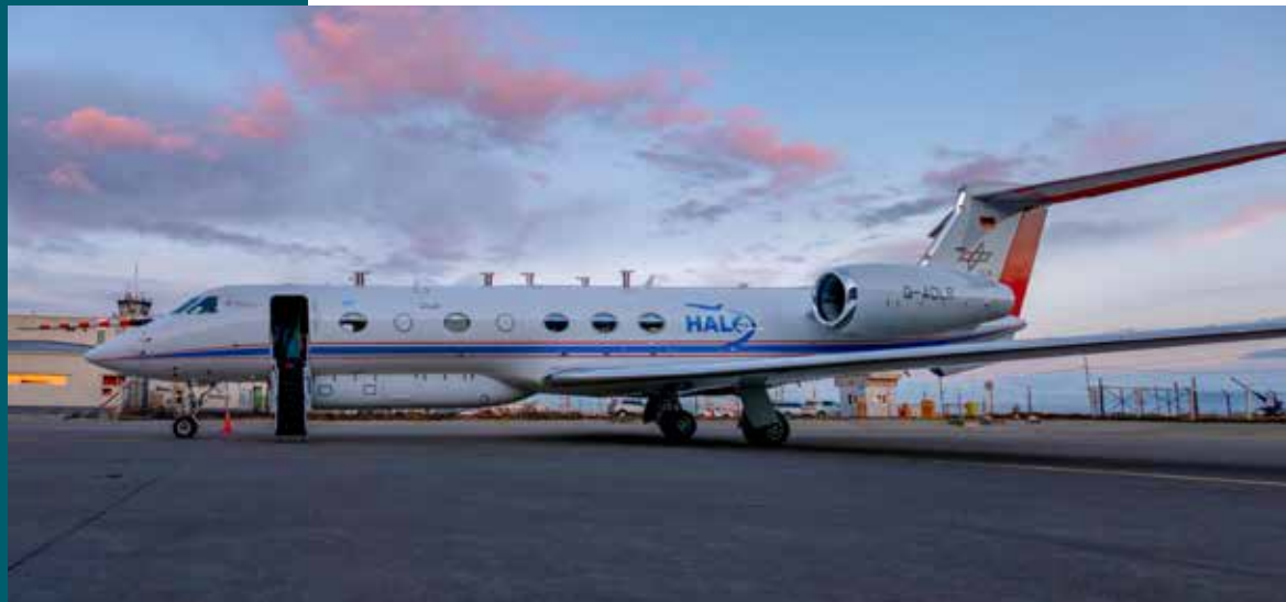
The HALO research aircraft on the apron of the airport in Río Grande. Inlets can be seen on the upper edge of the fuselage. Air is drawn through these into the interior of the cabin for analysis.
