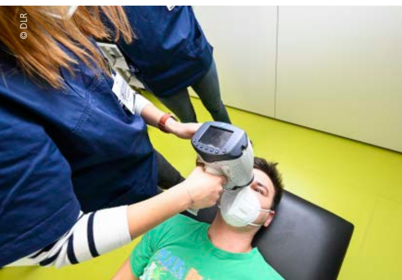
The change in the length of the eye axis is measured to rule out the contraction of the eyeball
