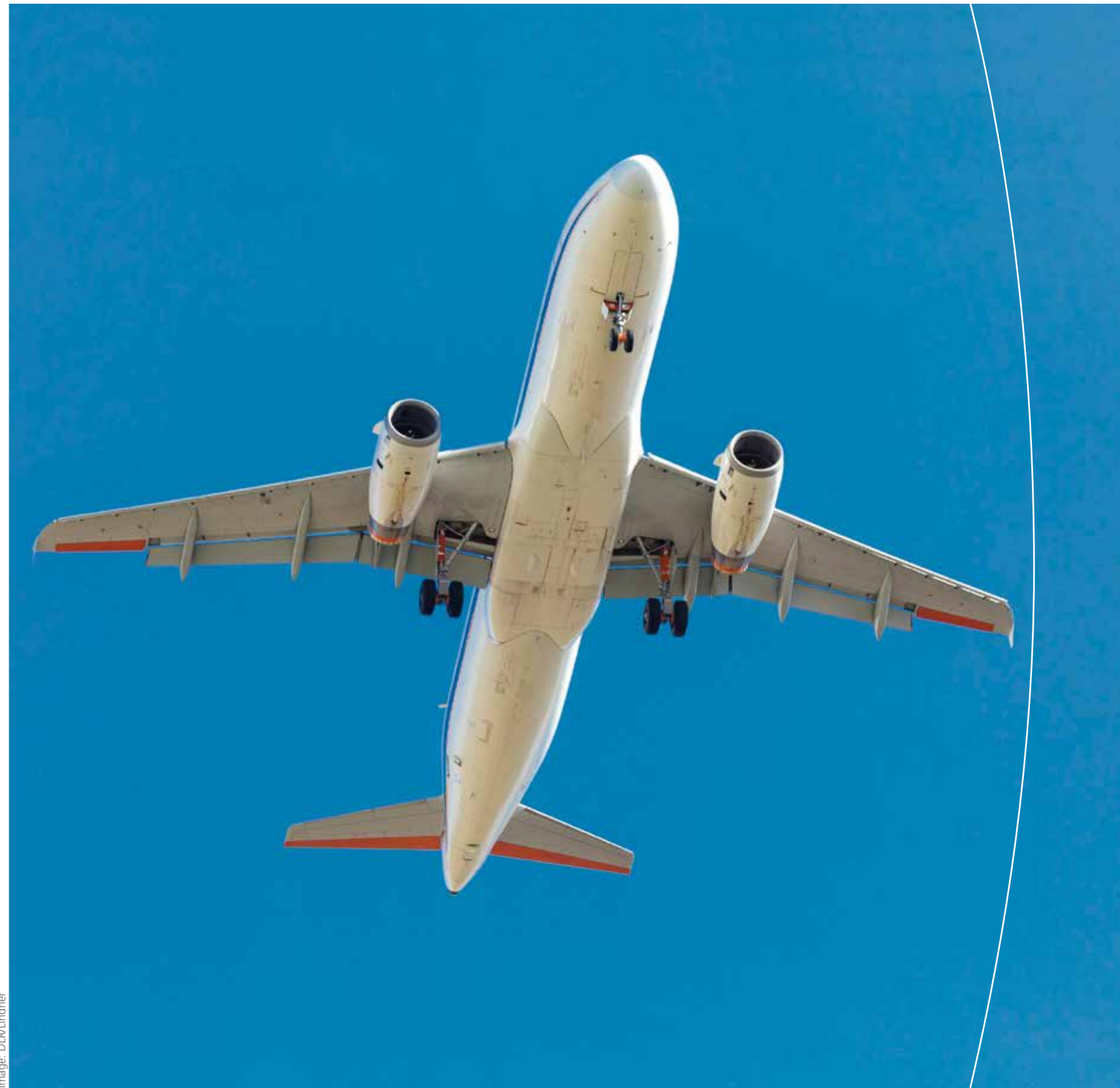
Low Noise ATRA: the modifications to the flaps, landing gear and engine exhausts – clearly visible in orange-red – should make flying quieter.
