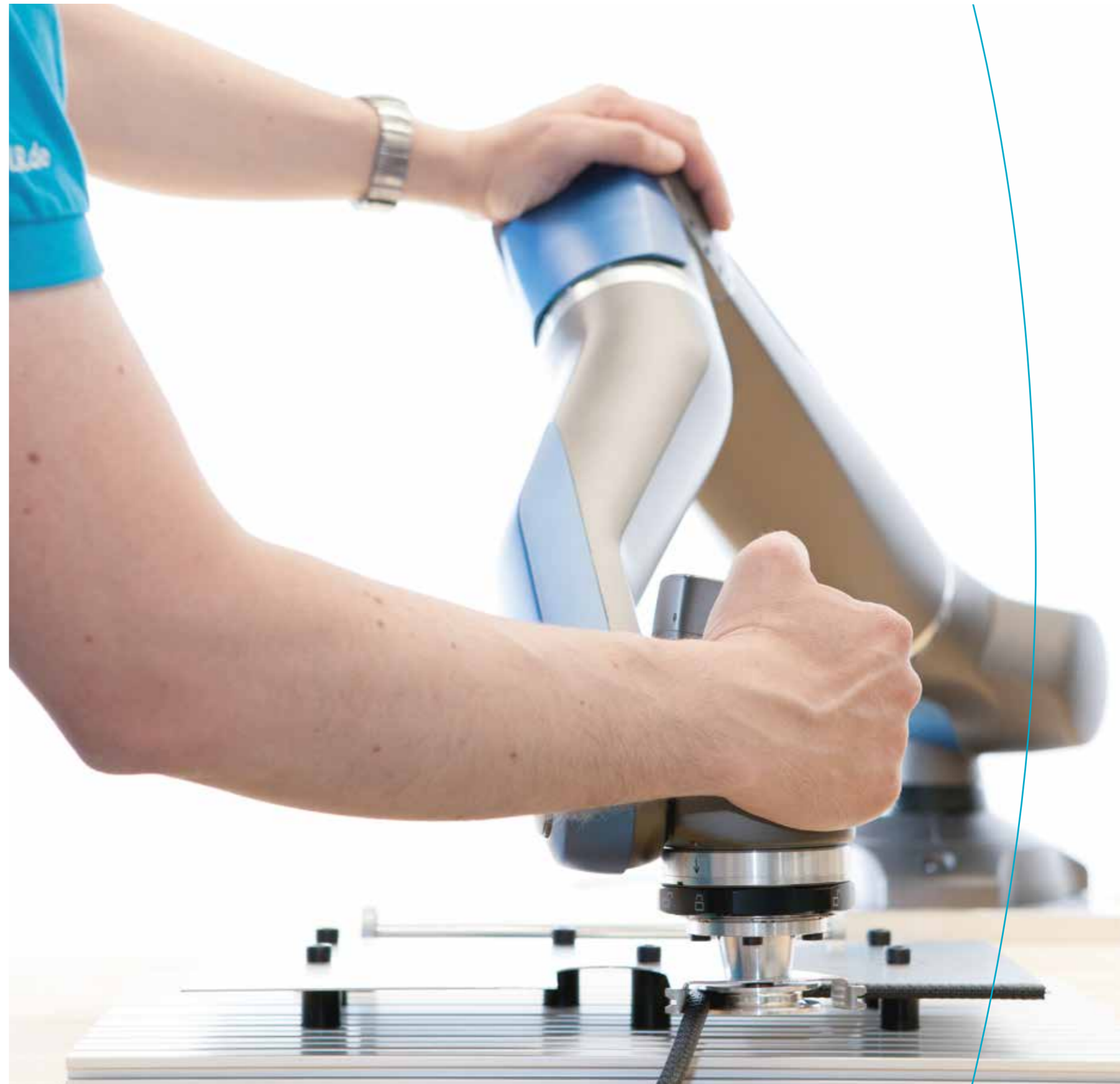
Programming through demonstration: The lightweight robot SARA learns from its human operator, who not only shows the robot what task it should perform, but also how it should be performed.
