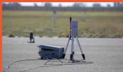
Storage and radio control unit for the operation of two widely dispersed field microphones
