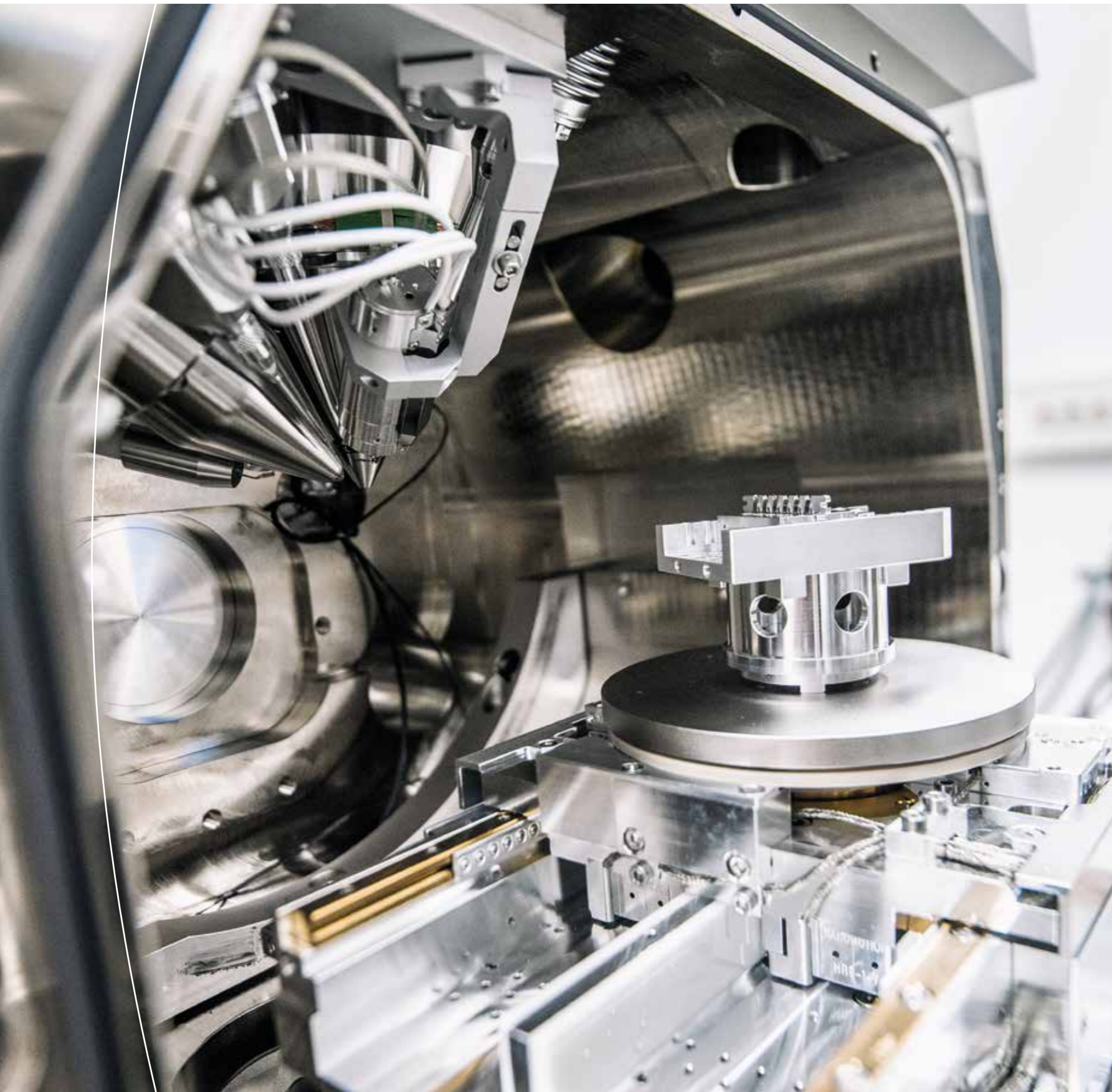
A view inside the focused ion beam microscope, in which an ion beam can perform miracles.
