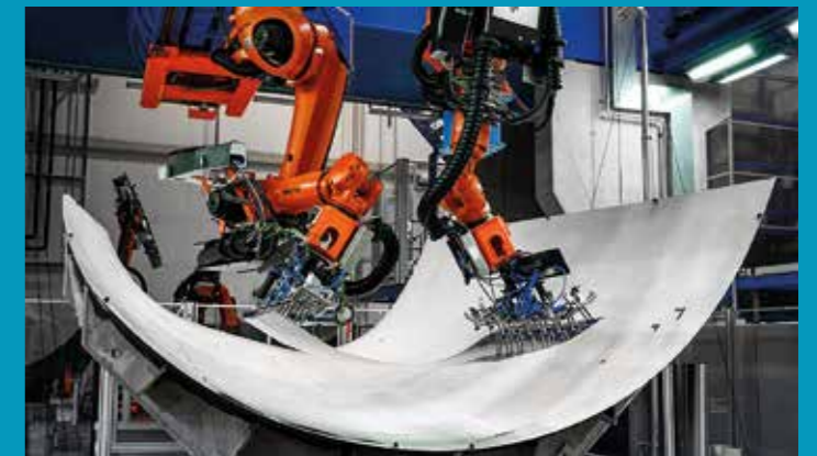
Robots lay aluminium sheets at ZLP Augsburg
