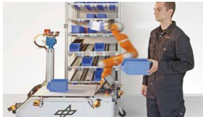
The robot will choose its working location in the future. To do so, it must be able to perceive its environment, plan its trajectories and identify objects.
