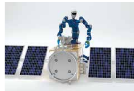
A service robot like the humanoid Justin can reproduce the arm and head movements of the service engineer
