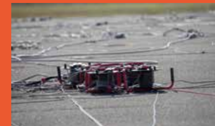
Cable drums for supply and data cable connections to microphones in the ground array (background)
