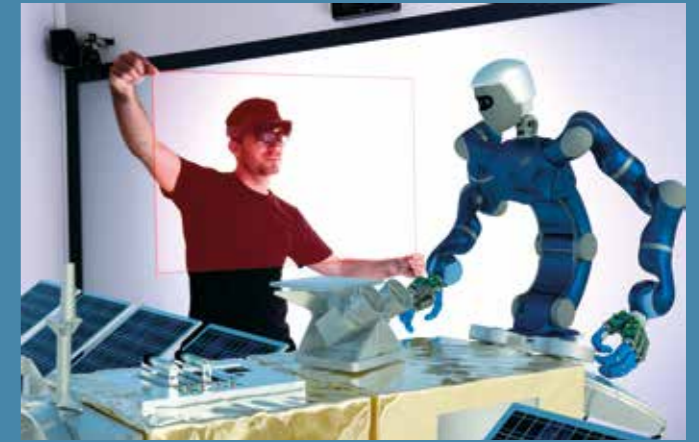
The expert draws up a barrier with his hands, and the robot knows it cannot move further.
