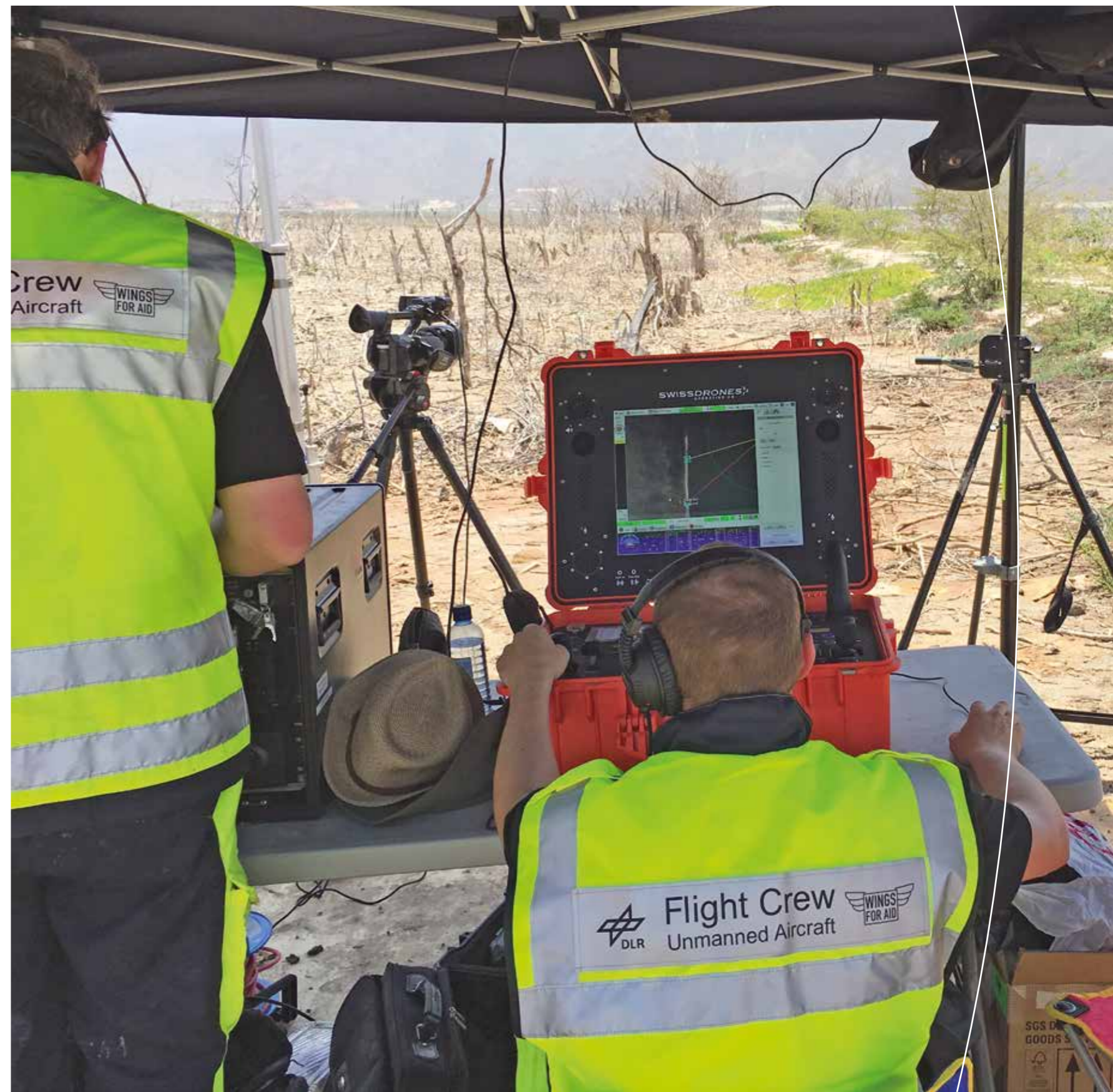
The ground station is like a camp, but has everything the crew needs to track the autonomous flying helicopter.
