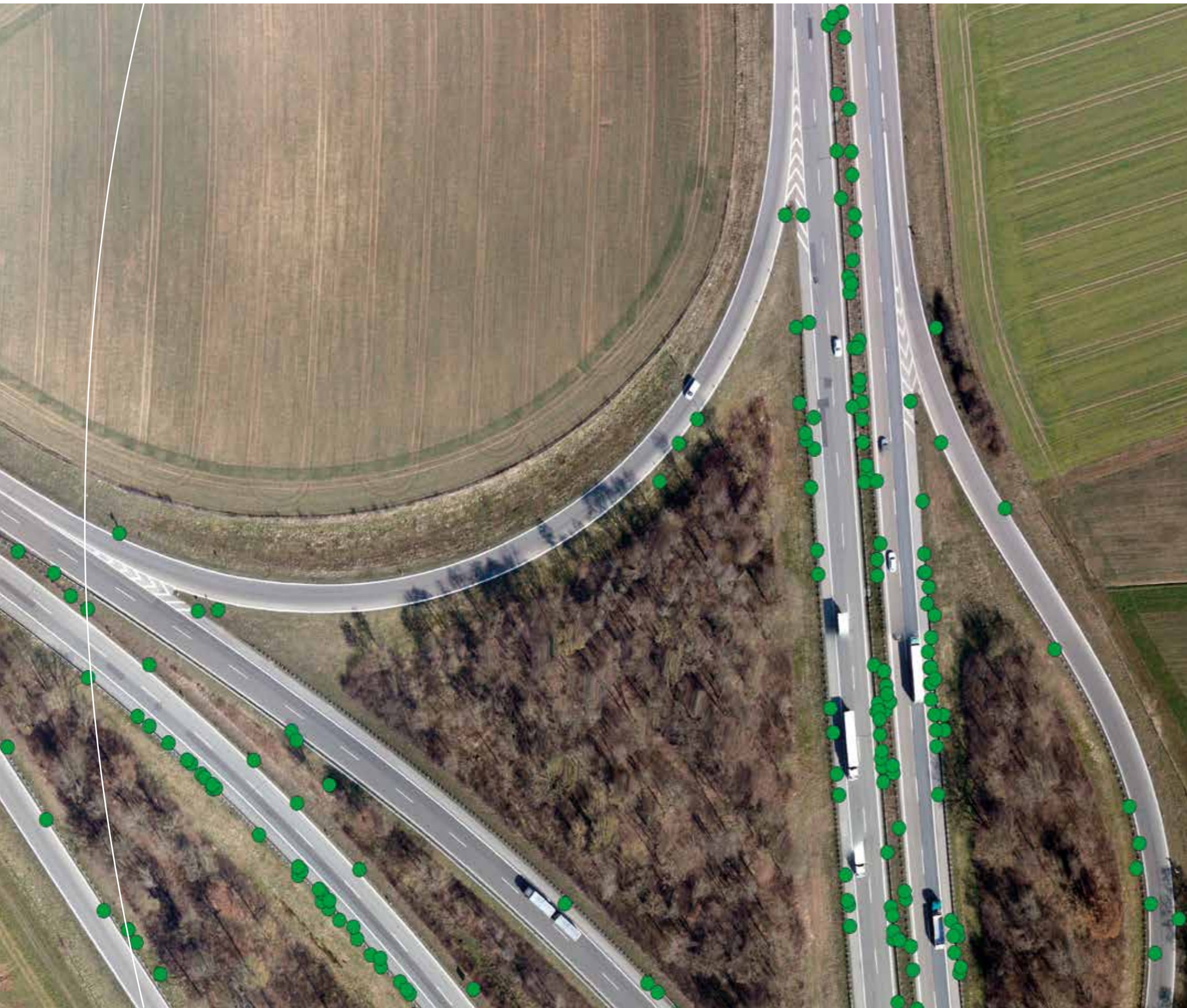
Capturing the road environment accurately in an image: The radar satellite TerraSAR-X records distinctive points on the roadside (DriveMarks), such as traffic signs and guardrail posts (here at the Hittistetten motorway junction near Ulm). The information about lane markings was acquired from aerial images provided by a DLR research aircraft equipped with the Institute's own 3K camera system.
