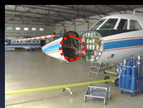
meteorological sensor package (temperature, pressure, humidity, wind)
