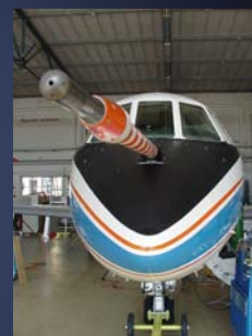
nose boom with flow angle sensor (CFK, 1.8 m length)
