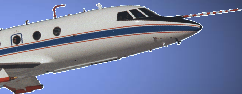
nose boom with flow angle sensor (CFK, 1.8 m length)
