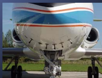
multiple temperature sensors and inlets for standard sensor package
