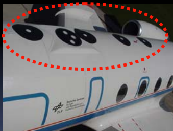
1 large opening on top of fuselage (515 mm diameter), (added in 1997)
