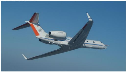
The HALO (High Altitude and LOng Range) research aircraft is based on the ultra-long-range G 550 business jet produced by Gulfstream Aerospace. With a range of more than 8000 kilometres, measurements on the scale of continents are possible; the research aircraft can reach all regions, from the poles to the tropics, and remote areas of the Pacific Ocean.
