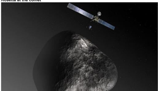
Artist's impression of the Rosetta spacecraft at its destination, Comet 67P/Churyumov-Gerasimenko. The picture is not to scale; the spacecraft's solar arrays have a span of 32 metres; the diameter of the nucleus is about four kilometres.
