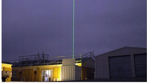
A mobile DLR LIDAR, which is housed in a container at NIWA's Lauder Atmospheric Research Station, also serves as an information source for studying gravity waves in the mesosphere.
