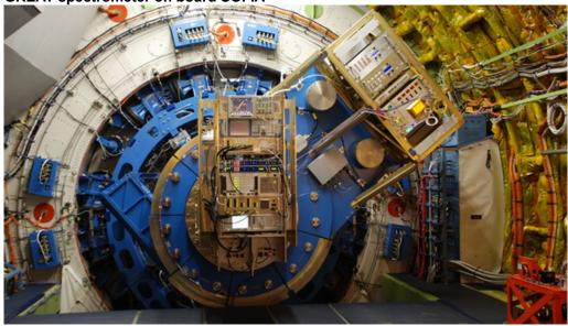
The GREAT far-infrared spectrometer (the vertical structure in the foreground) is mounted to the telescope counterweight flange inside the pressurised cabin. During observations, GREAT rotates ±20 degrees from the vertical, while the telescope (invisible on the far side) and its counterweight (seen here in blue at an angle of 45 degrees) move between roughly 25 and 65 degrees from the vertical.
