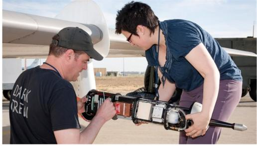
Installation of a measurement probe. Particulate measurement probes are installed under the wing of the Falcon. Here, one of the probes is being maintained before it is used again.
