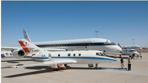
DLR Falcon and NASA DC-8. During the research flights, a NASA DC-8 led to the flight formation and burned different fuels. The DLR Falcon and a NASA Falcon followed the DC-8 at a distance of about 100 metres and collected data on the composition of the exhaust gases.
