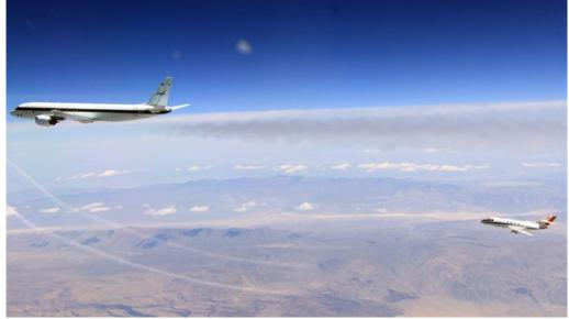
Behind the DC-8, the scientists on board the DLR Falcon measured the exhaust gas composition.
