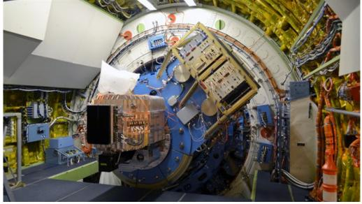
The image shows the rectangular aluminium cryostat of the FIFI-LS instrument mounted on the telescope's blue supporting structure. The cryostat is filled with liquid nitrogen and liquid helium for cooling the optical elements and detectors to the required low temperatures. The dark-coloured boxes in front of and below the cryostat and the obliquely arranged 'instrument rack' above are the electronic boxes for control of FIFI-LS and data processing.
