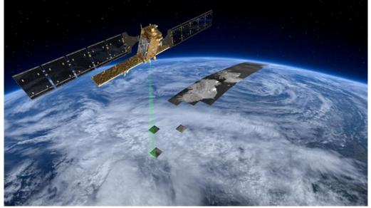
The Sentinel-1A satellite is quite flexible; the SAR sensor will operate in two main modes: Interferometric Wide Swath and Wave. The Interferometric Wide Swath mode is typically used for land surfaces and the Wave mode over oceans.
