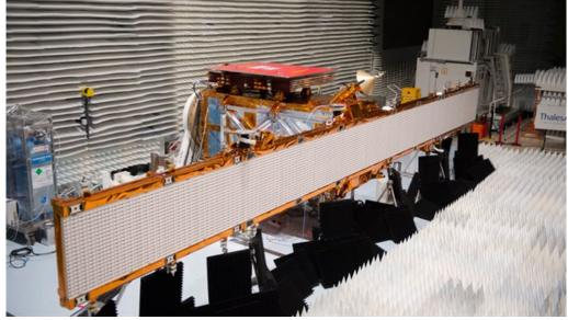
In the test chamber, Sentinel-1A is subjected to frequency tests. The 12-metre radar antenna can be seen in the centre of the image.
