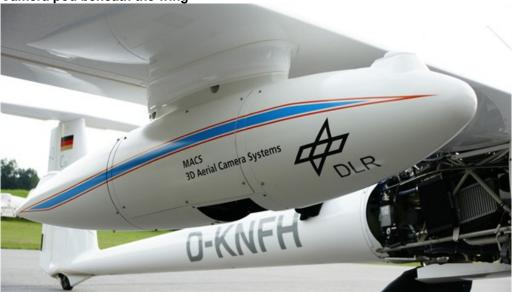
The Modular Aerial Camera System (MACS), a specialised apparatus developed and built by DLR, is fitted in an unpressurised instrument container mounted beneath the wing.
