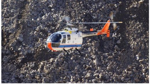
The Göttingen-based researchers employed a novel technique to visualise the rotor blade vortices, using the loose scree littering the quarry as a background for their measurement method.
