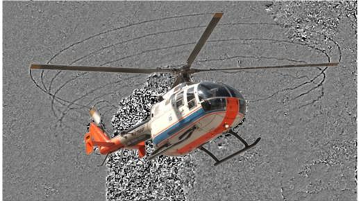
Blade tip vortices are visible as dark lines during a full rotation of the main rotor. The engine exhaust flows are perceptible as a noisy area trailing the helicopter. The tail rotor's vortex system is also visible (black, circular lines on the tail rotor). The helicopter is currently performing a rocking manoeuvre.
