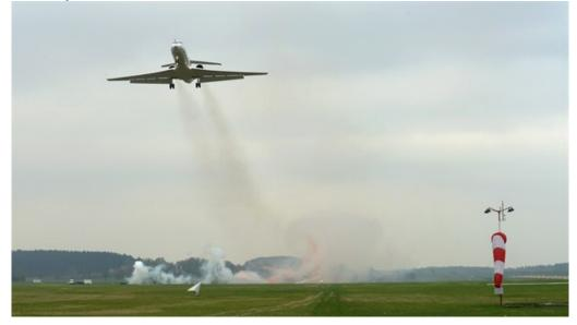
HALO fly-over: At 22 metres high, HALO flies over the experiment. In the smoke, the two wake vortices are visible.
