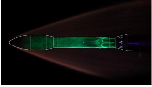
To record the change in air flow, renowned scientists conducted tests on a model of the Vega rocket in the wind tunnel at DLR in Cologne in June 2013. The images show the distribution of the oil particles during the different experimental conditions.
