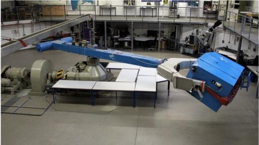
Candidates sit in a sealed cabin attached to a six-metre structure in the long-arm centrifuge at the German Aerospace Center (DLR)
