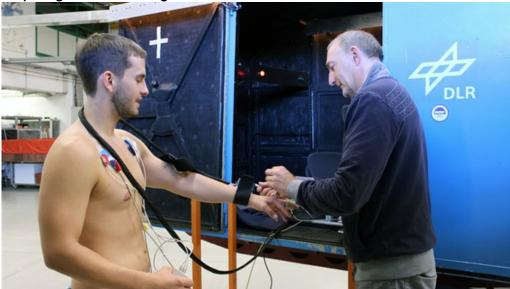
Peter Gauger from the German Aerospace Center (DLR) wires up the candidates before they get into the long-arm centrifuge, allowing the scientists to measure factors such as blood pressure and heart rate during the ride.
