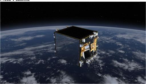
The European Proba-V satellite is also carrying a German Aerospace Center (Deutsches Zentrum für Luft- und Raumfahrt; DLR) payload. The receiver will locate the ADS–B (Automatic Dependent Surveillance – Broadcast) signals that flights transmit with a special antenna, while the satellite orbits Earth at an altitude of 820 kilometres.
