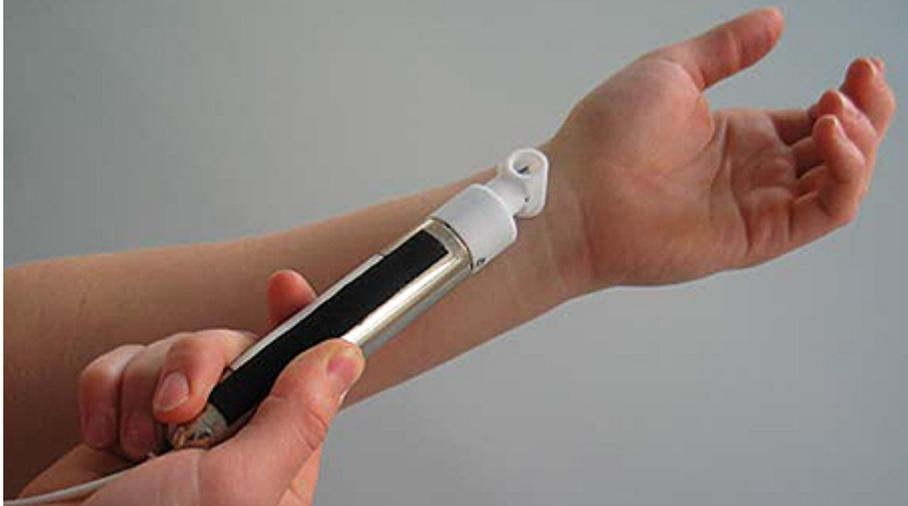
A Tewameter® being used to measure water loss from the skin. The measuring probe is part of the SKIN B experiment on the ISS. This will investigate the effect of microgravity on human skin.
