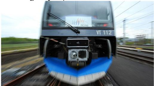
In the Railway Collision Avoidance System (RCAS) research project, DLR researchers have developed a complete system for preventing train collisions, which does not rely on any fixed infrastructure. The Bayerische Oberlandbahn (BOB) is a collaborative partner, having made one of its 'Integral' type regional trains, shown in this image, available as a test vehicle for RCAS. The technology is now ready for the market.
