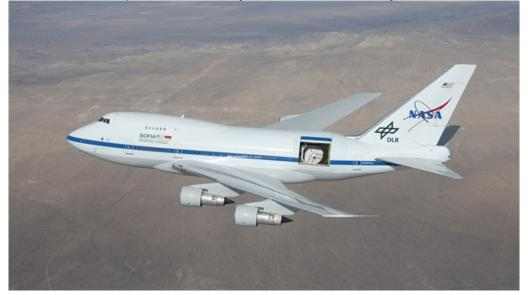
The Stratospheric Observatory For Infrared Astronomy (SOFIA) on its maiden test flight with a completely opened telescope hatch on 18 December 2009 over the Californian Mojave Desert. The 2.7 metre telescope, built in Germany, is visible through the opening in the fuselage of this Boeing 747SP. The test flight with an open hatch enabled engineers to examine the movement of air in and around telescope and door under experimental conditions for the first time.
