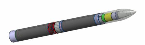
The VLM-1 is a small satellite launcherwhich is to be qualified for its first space mission by the Brazilian space agency, AEB. In 2016, VLM will to carry the SHEFEX-3 (SHarp Edge Flight EXperiment) spacecraft to the region between the upper layers of the terrestrial atmosphere and space. SHEFEX-3 will then separate from the VLM and return autonomously to the Earth at a velocity of seven kilometres per second.
