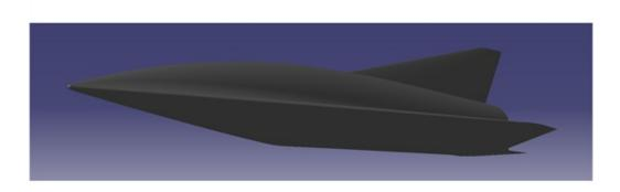
The SpaceLiner is a revolutionary concept on the boundary between air travel and spaceflight. With this ultrafast glider, passengers are expected to be able to cover the distance between Europe and Australia in just 90 minutes. The concept is based on an environment-friendly rocket engine that uses hydrogen and oxygen.
