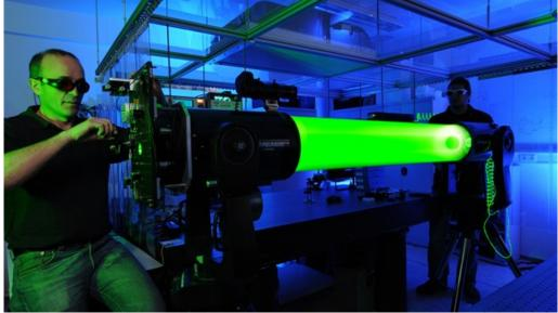
The Institute of Technical Physics at the German Aerospace Center (Deutsches Zentrum für Luft- und Raumfahrt; DLR) develops and builds lasers. In the future, lasers will be capable of detecting items of space debris and accelerating the decay of their orbits.
