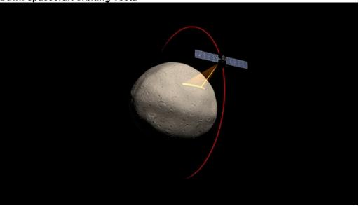
NASA's Dawn spacecraft, powered by ion propulsion, is carrying three different instruments to the main asteroid belt between Mars and Jupiter. Alongside a spectrometer from the Italian space agency (Agencia Spaziale Italia; ASI) and a gamma ray and neutron detector from the Los Alamos National Laboratory, is a German camera system, referred to as a 'framing camera', on board.
