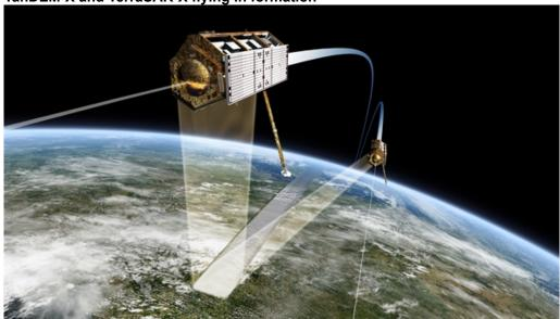
Flying in formation, TanDEM-X and TerraSAR-X will generate a precise global elevation model. Credit: DLR.
