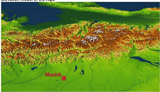
This elevation model was derived from the differences between two radar images acquired by the ESA satellites ERS-1 (European Remote Sensing-1) and ERS-2.
