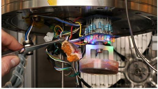
In the Mars simulation chamber, DLR researchers recreated the atmospheric composition and pressure, the planet's surface, the temperature cycles and the solar radiation incident on the surface. The activity of polar and alpine lichen was investigated under these conditions.
