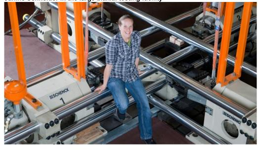
Janine Schneider with the largest test bench for mechanical materials testing, the large biaxial testing facility.
