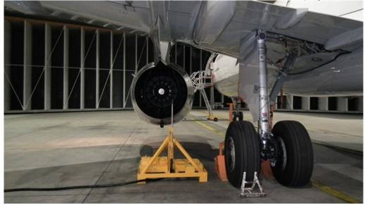
These tests were conducted during the night at Hamburg's Fuhlsbüttel Airport, and involved ground simulations of the various phases of a flight – take-off, steep ascents and final approach. The researchers conducted these probe measurements on both engines, which enabled them to compare the pollutant emissions of a 50-percent biokerosene mix with those from normal kerosene.
