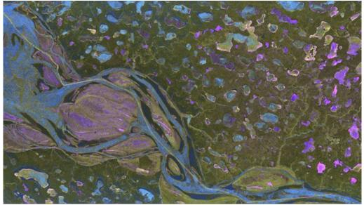
Radar signals from the TerraSAR-X satellite can penetrate the upper layers of snow and ice that cover the Mackenzie River in Canada. The shades of colour enable DLR researchers to draw conclusions about the ice formations and various subsurfaces.
