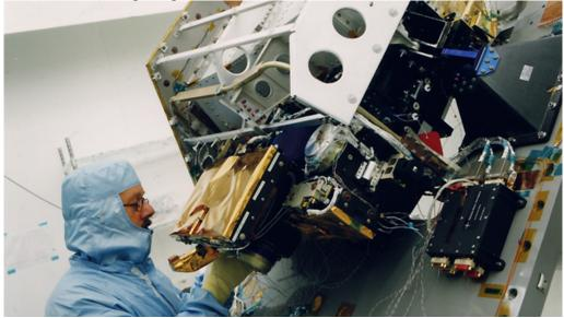
The German-Dutch-Belgian 'SCanning Imaging Absorption SpectroMeter for Atmospheric CartograpHY' – SCIAMACHY– during integration.
