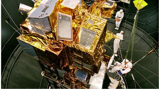
Envisat was extensively tested in the Large Space Simulator at ESA's ESTEC facility. In this image, Envisat is being prepared for thermal testing.
