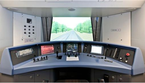
The DLR RailSiTe train laboratory enables detailed technical and operational simulations and testing of railway control and safety technology. It has now been accredited as the only German laboratory for testing components of the European Train Control System (ETCS).
