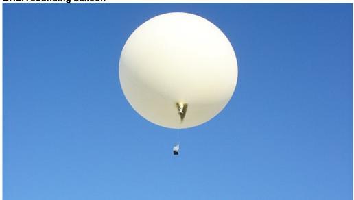
The sounding balloon is made of special rubber material and is about 1.50 metres in diameter. The balloon is filled with helium and can reach an altitude of 30 kilometres.
