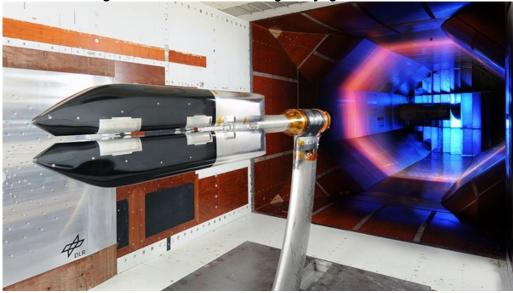
With this double-deck train model made from carbon-fibre-reinforced composite, DLR researchers measure, among other things, the noise emitted by a high-speed train.
