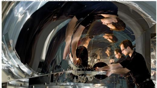
Using artificial sunlight, researchers use this test stand to investigate the optical, geometrical and mechanical quality of the mirrors that capture and concentrate the sunlight in a solar power station, as well as the properties of the pipes that absorb the energy and transfer it in the form of heat.
