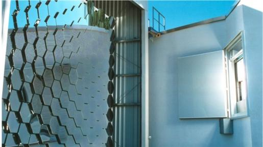
A 57 square metre mirror collects sunlight and directs it towards the facetted mirrors (left in the picture). These mirrors concentrate the incoming radiation up to around 5200 times and direct it to the research laboratory of the Cologne solar furnace (the beam of light can be seen on the right of the image).
