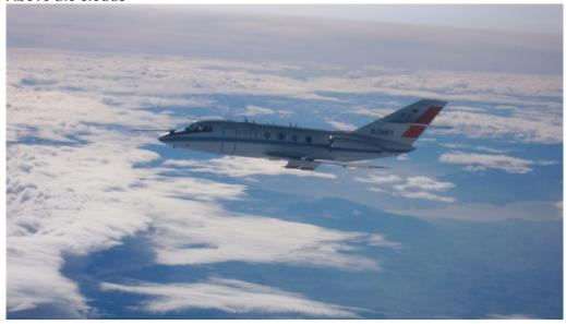
The Falcon 20E in flight. The DLR research aircraft can carry up to 1100 kilograms of scientific instrumentation payload. The instruments are installed inside and below the cabin, as well as under the wings. They include a flow measuring device, the nose boom, air intakes and underwing pods. Among other things, they include a flow measuring device, the so-called nose boom and antennas which can be mounted on the exterior of the aircraft.
