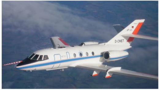
The DLR Falcon 20E research aircraft was selected as the most appropriate aircraft for measurement flights. The Falcon has a full range of instruments to record flight dynamics and a nose boom that records the local incidence angle at the front of the aircraft in an undisturbed airflow.
