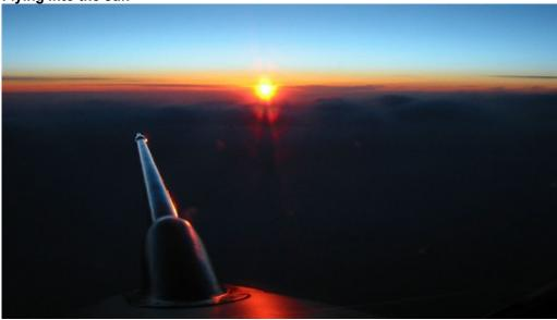
View from the cockpit of the Falcon during a research flight in 2002. The 1.8-metre nose boom has a five-hole sensor at its tip that provides scientists with very accurate information about, among other things, the static and dynamic pressure in the atmosphere.
