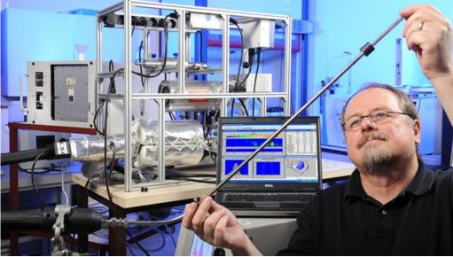
Claus Wahl, a DLR scientist in the Chemical Analysis Department, working on a mobile measuring device to analyse exhaust emissions and measure particulates generated by 'Gas to Liquid' (GtL) fuels. In modern combustion research, chemical and instrument analyses are indispensible in analysing the emissions from combustion processes and deriving measurements to reduce pollutants.
