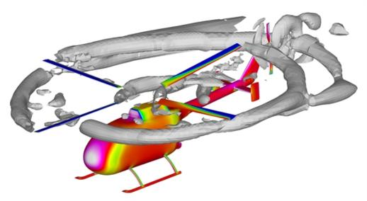
Reduced pressure on the top of the blade draws air upwards; this produces a vortex – the blade tip vortex – that is then directed downwards. When other rotor blades subsequently come into contact with these vortices, the 'chopping' or throbbing noise characteristic of helicopters is produced.
