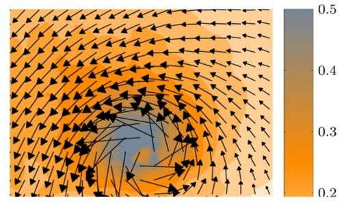
This measurement image shows the instantaneous velocity field in a rotor tip vortex.
