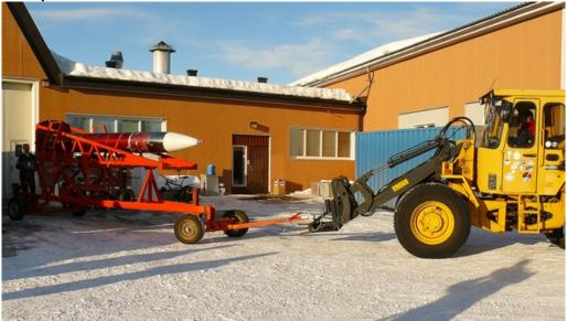
The TEXUS 49 payload being transported to the launch tower, where it is will be mated with the rocket.
