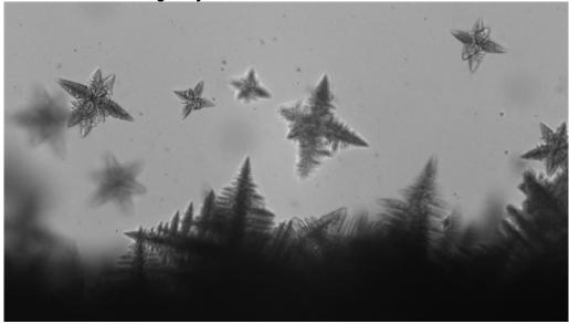
The TRACE+ experiment investigates the processes and structures involved in the solidification of metallic alloys. This is done by analysing the behaviour of a mixture of organic substances with a solidification process similar to that of a liquid metal. The transparency of the organic alloy made it possible to observe its solidification process directly.
