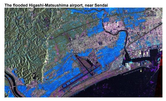
This radar image, acquired by the German Earth observation satellite TerraSAR-X on 12 March 2011 at 21:43 CET, shows the impact of the tsunami on Higashi-Matsushima Airport and the port of Ishinomaki, near Sendai, on the east coast of Japan. The blue areas indicate the flooding; the magenta-coloured areas show the extent of the destroyed infrastructure.
