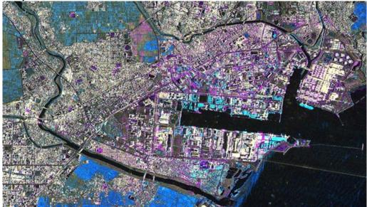
This TerraSAR-X image, acquired on 12 March 2011, shows that the port of the Japanese city of Sendai has been devastated by the tsunami. The magenta-coloured areas reveal the extent of damage in the form of boulders and debris deposits; the blue areas are flooded.
