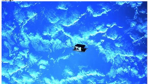
PRISMA is the first European satellite mission to demonstrate autonomous formation flying at distances between 30 kilometres and two metres. The main satellite, Mango, and its partner satellite, Tango, fly around one another in varying formations as they orbit the Earth. The satellites carry out orbit control and navigation independently.
